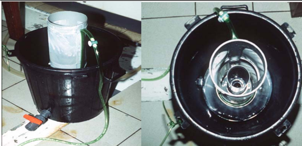
Figure 3.10. Side and upper view of a concentrator rinser containing a filter with a mesh size of 50 \mu\text{m} and equipped with an aeration collar at the bottom.
