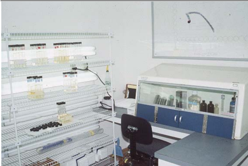
Figure 2.4. Temperature controlled room for maintenance of algal stock cultures in a bivalve hatchery: stock cultures in test tubes (left) and inoculation hood (right).
