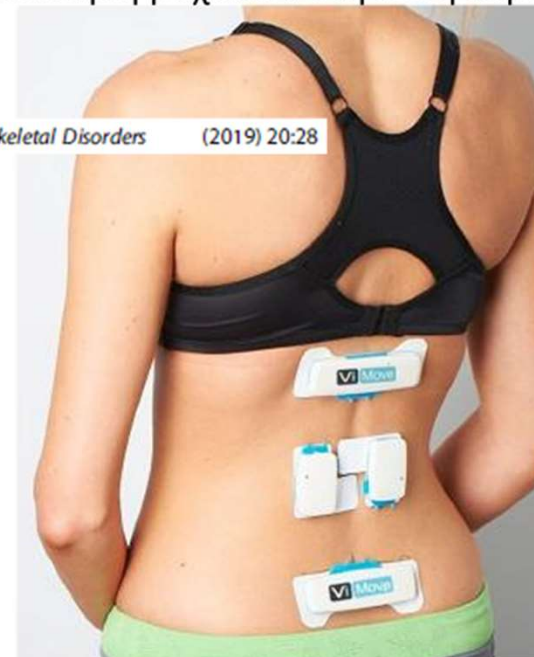
Fig. 1 Device Placement. An example of sensor placement with the lower border of the upper sensor placed at the T12 level, the upper border of the lower sensor level with S1 and the EMG sensors placed over lumbar extensor muscles at the level of L3
