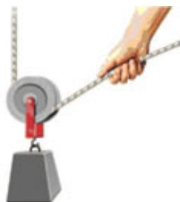
*Figure 3.* The movable-pulley arrangement used for the classroom demonstration.
