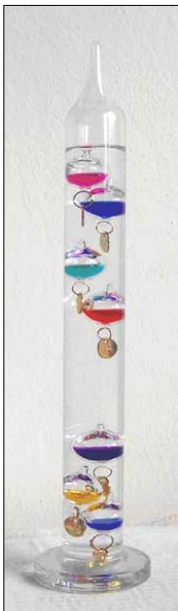
Figure 2. A Galileo thermometer.
