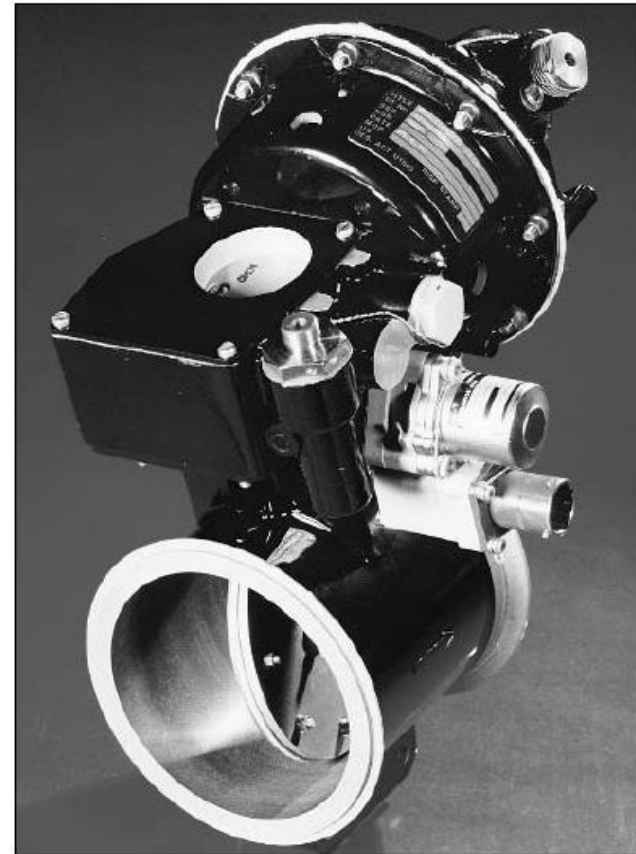
Harrier II pneumatic valve (Honeywell Normalair-Garret Ltd)
