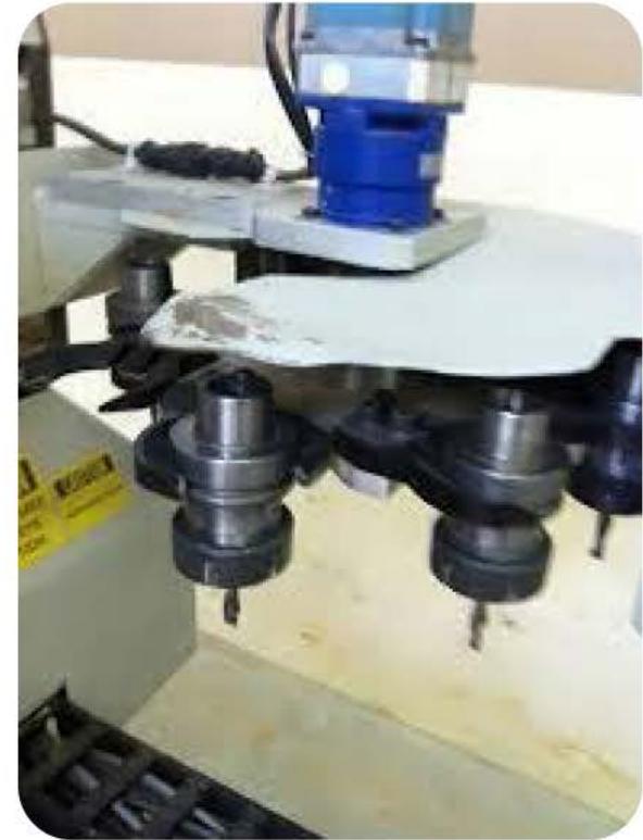
FIGURE 2 Tool Carousel on the MultiCAM
