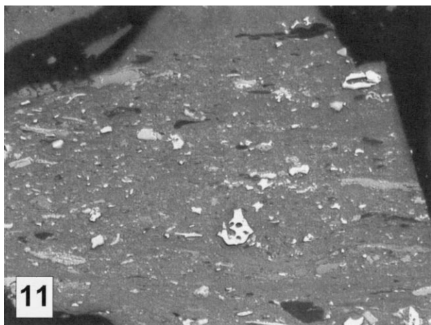
Fig. 11. Inertodetrinite (bigger white grains) and Micrinite (fine white grains); El Cerrejon Norte, Colombia; Tertiary.
