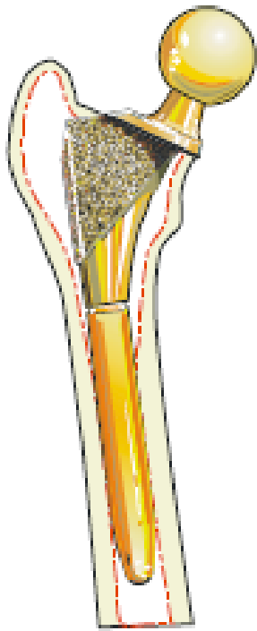
Use of a larger diameter extension with thin walled femoral shaft to obtain both a precise proximal flare and femoral shaft fit
