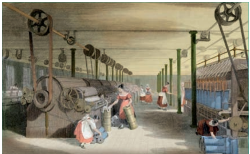
figure 2. Belts and pulleys—mechanical power transmission in the age of steam. (Source: http://ifsa.my/articles/mechanical-power-transmission-part-i-an-overview/ ; in the public domain.)
