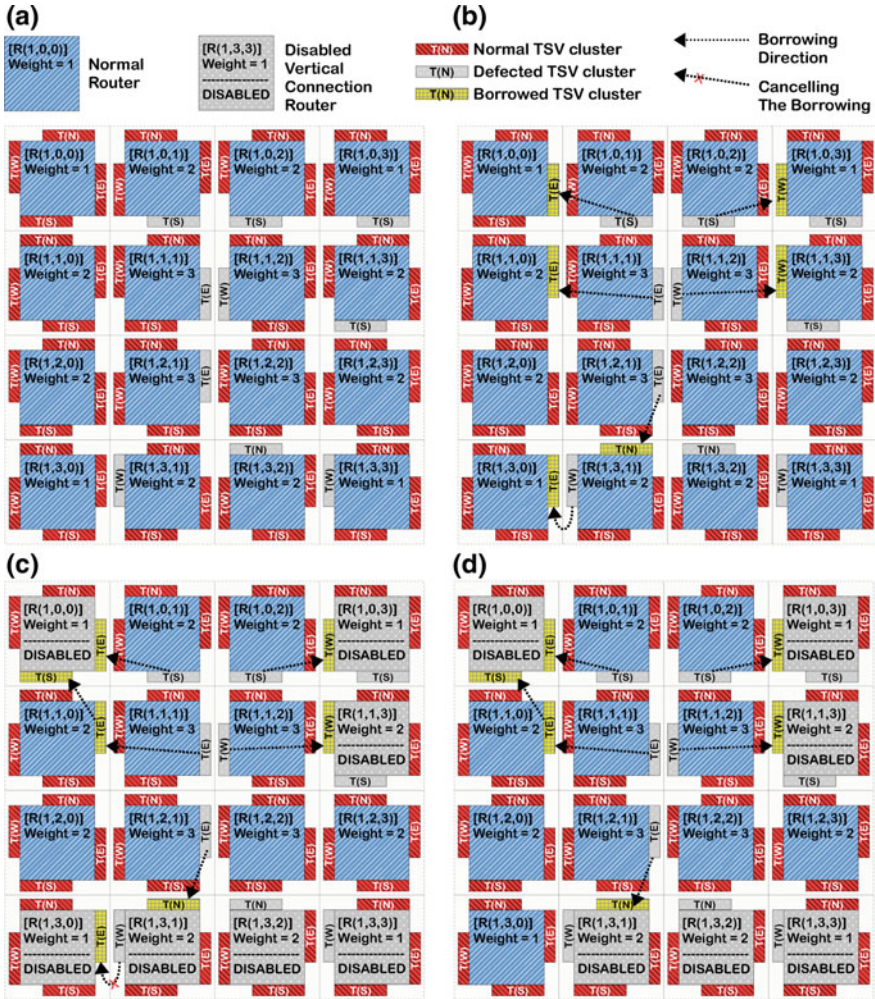
Fig. 6.8 An example of the sharing algorithm on a 4 \times 4 layer: a Initial state with ten defected TSV clusters; b Best candidates selection; c Borrowing chain creating and selection refining. d Final result with six disabled routers
