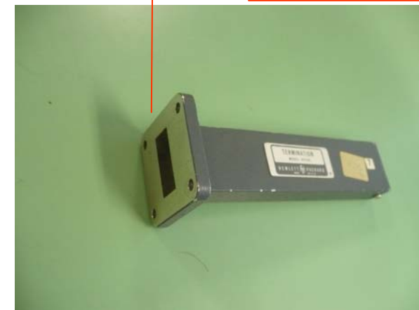
HP Termination No. H 910A
