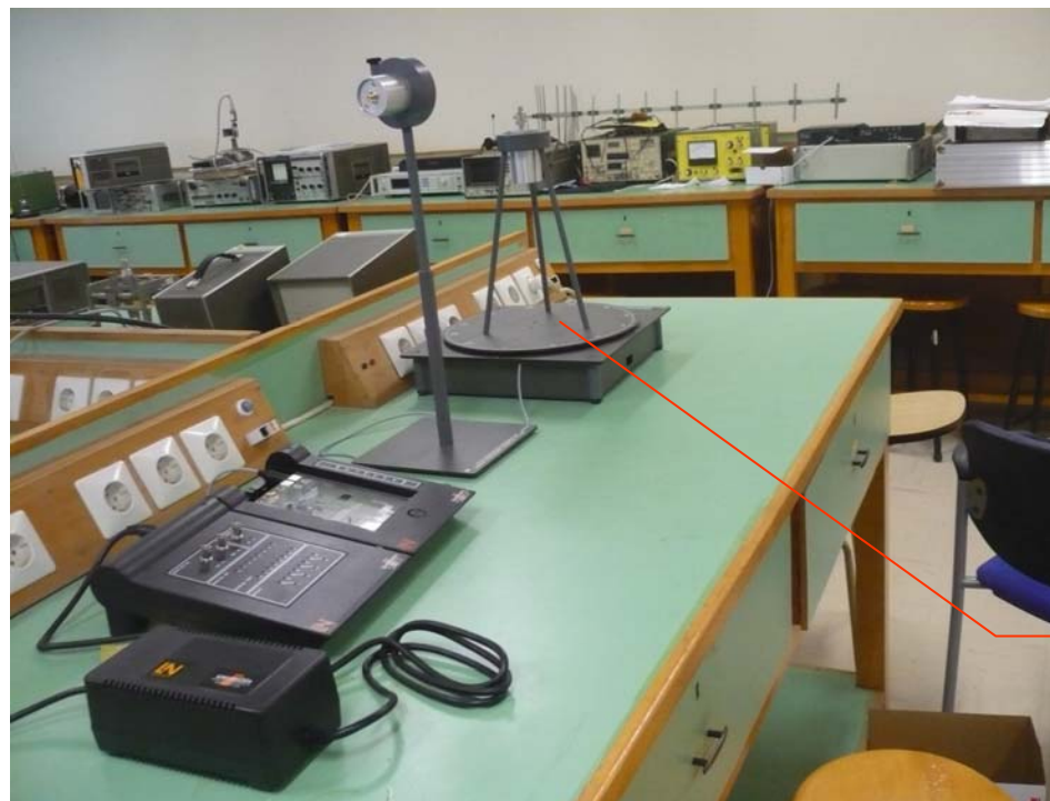
Antenna Positioner with stepper Motor
