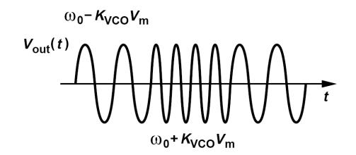
As an example, suppose  $V_{cont} = V_m \sin \omega_m t$ , i.e., the frequency of the oscillator is modulated periodically. Intuitively, we expect the output waveform frequency periodically swings between  $\omega_0 + K_{VCO}V_m$  and  $\omega_0 - K_{VCO}V_m$ , i.e., has a "peak deviation" of  $\pm K_{VCO}V_m$ . However, the student's expression yields
