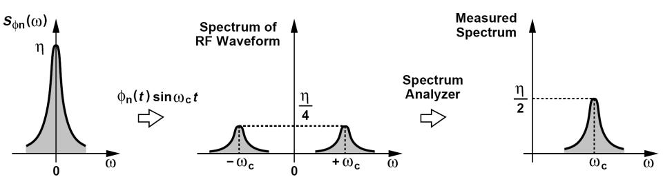
> (1) since  $\Phi_n(t)$  in equation above is multiplied by sin  $\omega_c t$ , its power spectral density,  $S_{\phi_n}$ , is multiplied by 1/4 as it is translated to  $\pm \omega_c$ ;
