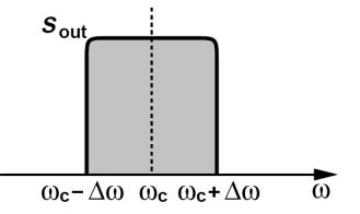
This spectrum occurs if the oscillator frequency has equal probability of appearing anywhere between  $\omega_c - \Delta \omega$  and  $\omega_c + \Delta \omega$ . However, we intuitively expect that the oscillator prefers  $\omega_c$  to other frequencies, thus spending lesser time at frequencies that are farther from  $\omega_c$ . This explains the declining phase noise "skirts".
