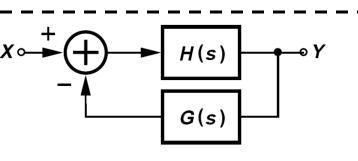
If the feedback path has a transfer function G(s), then  $|\frac{Y}{X}(j\omega_0 + j\Delta\omega)|^2 = \frac{1}{4Q^2} \left(\frac{\omega_0}{\Delta\omega}\right)^2 |\frac{1}{G(j\omega_0)}|^2$   $Q = \frac{\omega_0}{2} |\frac{d(GH)}{d\omega}| \qquad 36$
