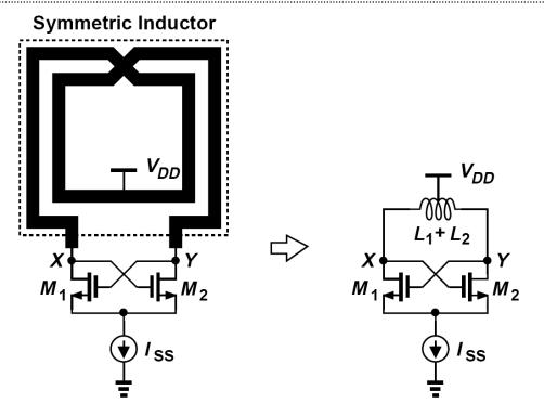
The symmetric inductor above has a value of 2 nH and a Q of 10 at 10 GHz. What is the minimum required transconductance of  $M_1$  and  $M_2$  to guarantee start-up?
