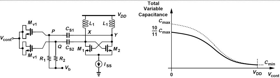
The principal drawback of the above circuit stems from the parasitics of the coupling capacitors.
