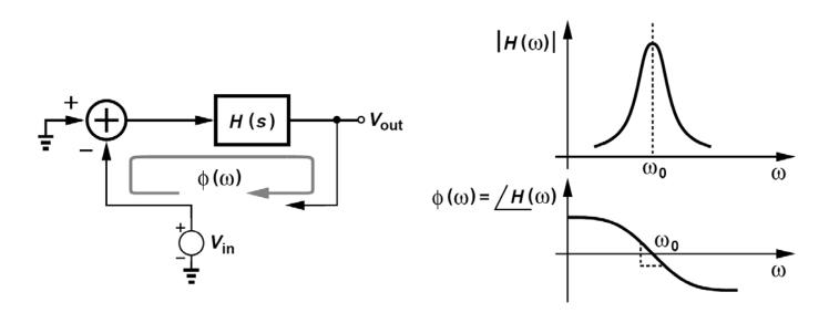
Another definition of the Q that is especially well-suited to oscillators is shown above, where the circuit is viewed as a feedback system and the phase of the open-loop transfer function, is examined at the resonance frequency.
