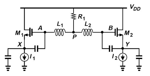
If chosen properly, the resistor  $R_1$  prohibits common-mode oscillation.
