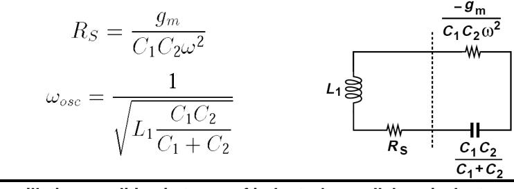
Express the oscillation condition in terms of inductor's parallel equivalent resistance,  $R_p$ , rather than  $R_s$ .
