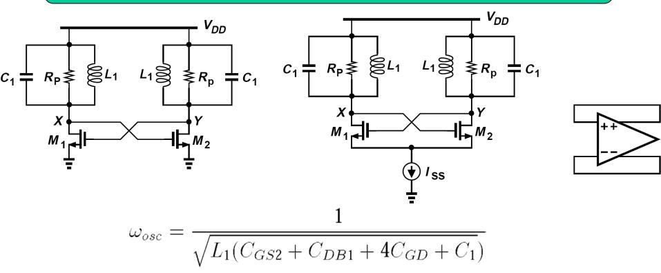
The oscillator above (left) suffers from poorly-defined bias currents. The circuit above (middle) is more robust and can be viewed as an inductively-loaded differential pair with positive feedback.
