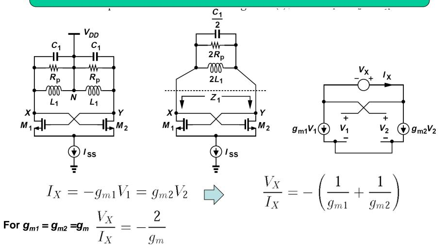
For oscillation to occur, the negative resistance must cancel the loss of the tank:
