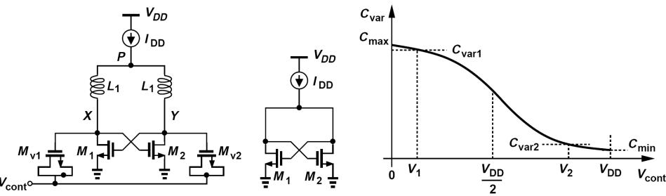
The CM level is simply given by the gate-source voltage of a diode-connected transistor carrying a current of  $I_{DD}/2$ .
