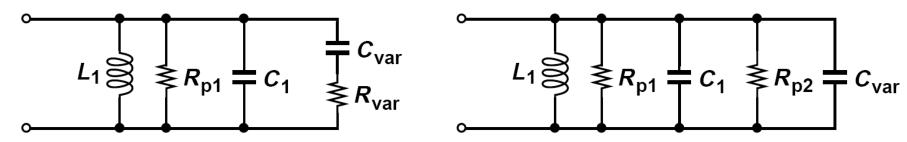
Transforming the series combination of  $C_{var}$  and  $R_{var}$  to a parallel combination
