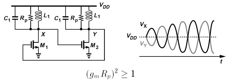
Assuming that the circuit above (left) oscillates, plot the voltage waveforms at *X* and *Y*.
