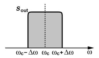
This spectrum occurs if the oscillator frequency has equal probability of appearing anywhere between  $\omega_c$  -  $\Delta\omega$  and  $\omega_c$  +  $\Delta\omega$ . However, we intuitively expect that the oscillator prefers  $\omega_c$  to other frequencies, thus spending lesser time at frequencies that are farther from  $\omega_c$ . This explains the declining phase noise "skirts".
