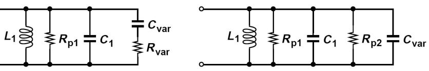
Transforming the series combination of  $C_{var}$  and  $R_{var}$  to a parallel combination
