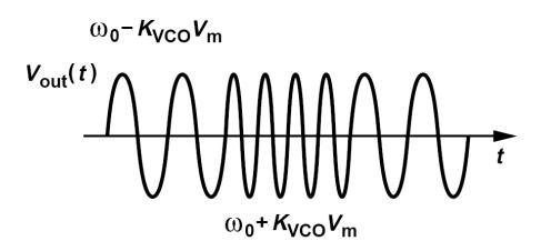
As an example, suppose  $V_{cont} = V_m \sin \omega_m t$ , i.e., the frequency of the oscillator is modulated periodically. Intuitively, we expect the output waveform frequency periodically swings between  $\omega_0 + K_{VCO}V_m$  and  $\omega_0 - K_{VCO}V_m$ , i.e., has a "peak deviation" of  $\pm K_{VCO}V_m$ . However, the student's expression yields
