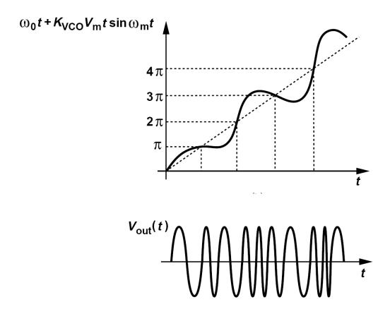
The intersection of each horizontal line with the phase plot signifies the zero crossings of  $V_{out}(t)$ . Thus,  $V_{out}(t)$  appears as shown above. The key point here is that the VCO frequency is not modulated periodically.
