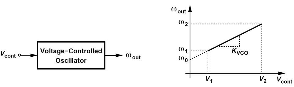
The output frequency varies from  $\omega_1$  to  $\omega_2$  (the required tuning range) as the control voltage,  $V_{cont}$ , goes from  $V_1$  to  $V_2$ .
