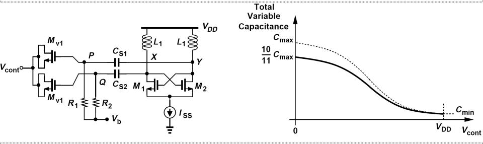
The principal drawback of the above circuit stems from the parasitics of the coupling capacitors.
