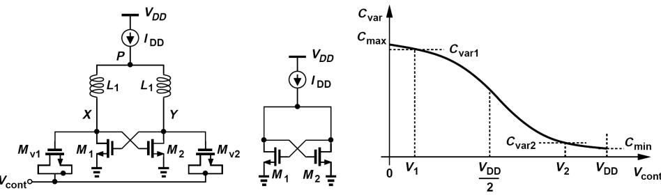
The CM level is simply given by the gate-source voltage of a diode-connected transistor
