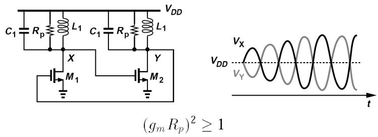
Assuming that the circuit above (left) oscillates, plot the voltage waveforms at *X* and *Y*.
