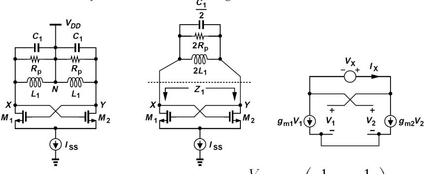
$$I_X = -g_{m1}V_1 = g_{m2}V_2$$
