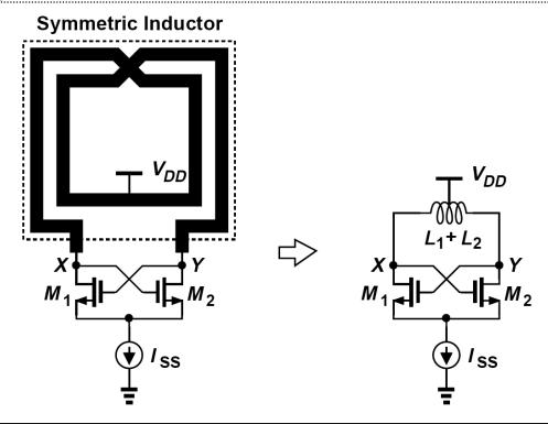
The symmetric inductor above has a value of 2 nH and a Q of 10 at 10 GHz. What is the minimum required transconductance of  $M_1$  and  $M_2$  to guarantee start-up?
