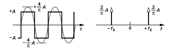
Recall from the Fourier expansion of a square wave of peak amplitude A (with 50% duty cycle) that the first harmonic exhibits a peak amplitude of  $(4/\pi)A$  (slightly greater than A). The peak single-ended output swing therefore yields a peak differential output swing of
