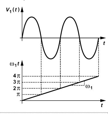
A VCO is simply a frequency modulator. For example, the narrow-band FM approximation holds here as well.
