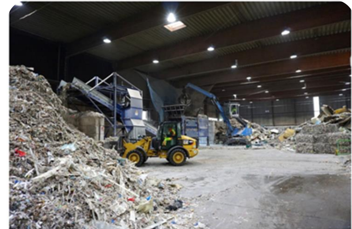
In a multi-stage process, the plant breaks up GFRPs and then combines them with paper production residue to create a raw material for cement
