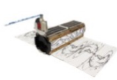
PlanetScope (Dove) Launch Mass 4kg
