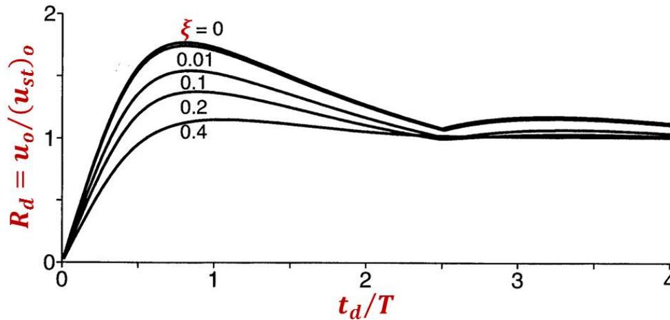
FIGURE: Shock spectra for a half-cycle sine pulse force for five damping values
