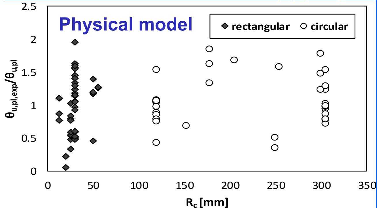
No apparent need for a lower limit of more than ~15 mm on FRP radius as far as its effect on failure of columns with lap-spliced bars is concerned.
