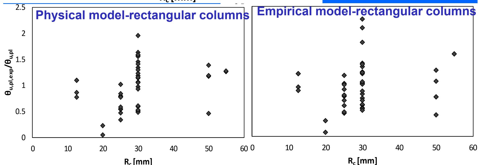
Members with smooth (plain) bars, continuous or lap-spliced (with hooks or straight ends), without or with FRP wrapping
