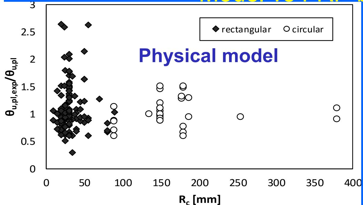
No apparent need for a lower limit more than  $\sim 15$  mm on the FRP corner radius, as far as its effect on column failure is concerned.
