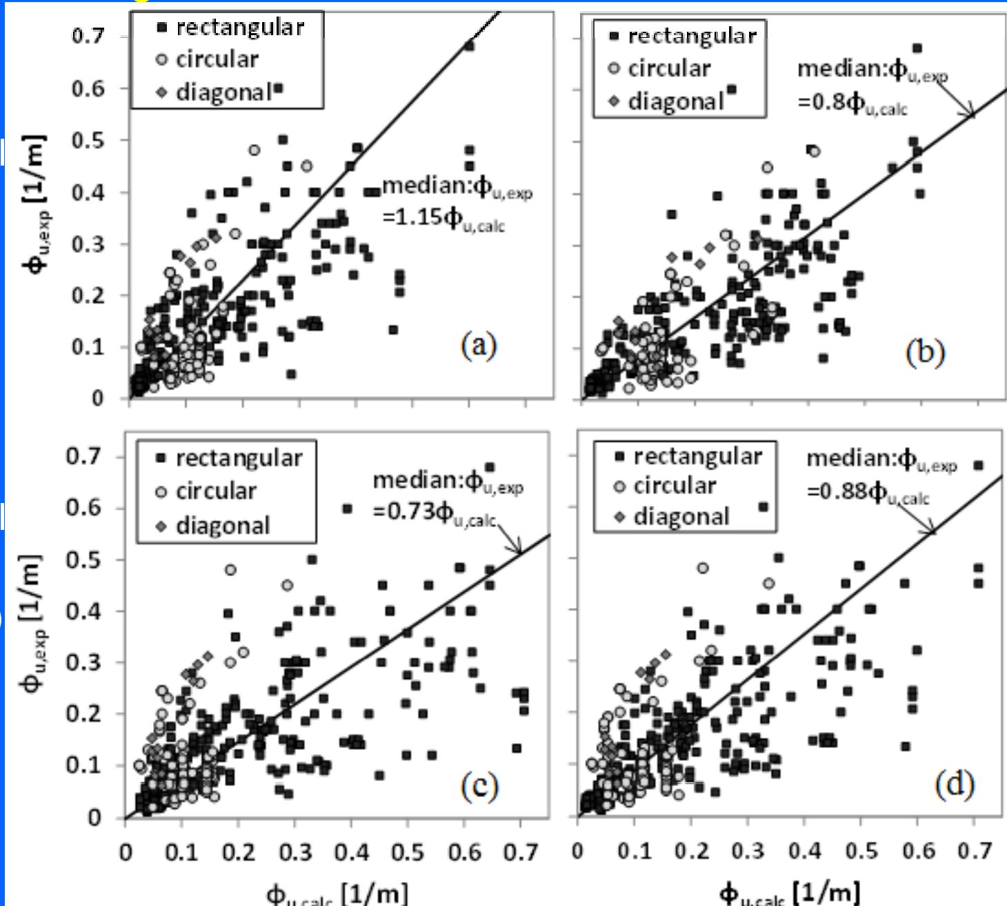
(645) measured ultimate curvatures in (410) tests vs values calculated using ultimate strains from Grammatikou et al 2016
