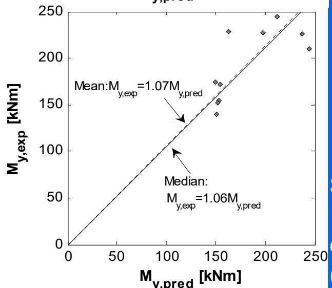
20 cantilever/double cantilevers laps & straight ends
