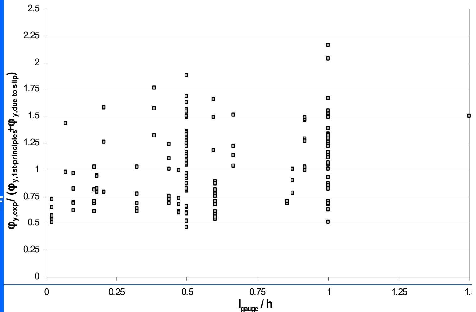
Fixed-end rotation of member end due to ribbed bar pull-out from yield penetration length in zone beyond the member end, at member **ultimate curvature**
