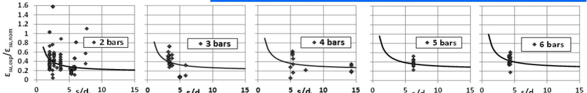
(374) measured ultimate curvatures from (184) cyclic tests vs values calculated using ultimate strains from current seismic codes
