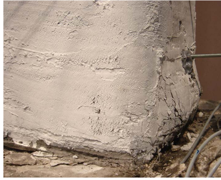
Fig. 7. Lateral expansion of TRM jackets at the base of RC columns without fiber rupture
