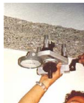
Fig. 7.14 In-situ testing of substrate strength.
