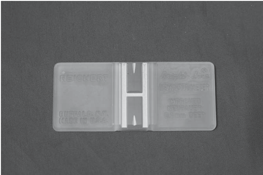
Figure 14.2. A hemacytometer. Photograph provided with the kind permission of WineBugs LLC.
