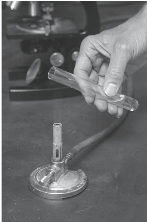
Figure 13.2. Heating the neck of a test tube prior to transfer of liquid. Photograph provided with the kind permission of WineBugs LLC.
