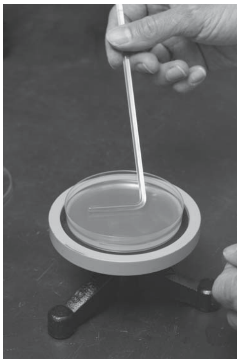
Figure 14.4. A glass “hockey stick” being used to spread a liquid sample over the surface of solidified agar. Photograph provided with the kind permission of WineBugs LLC.
