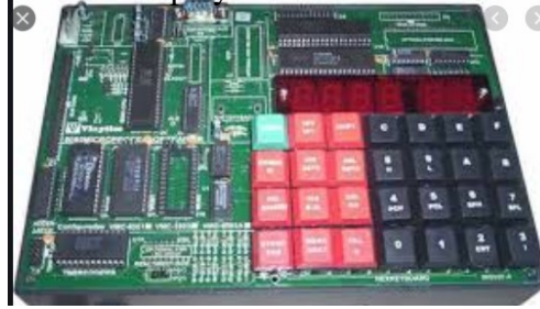
8085 Microprocessor Trainer Kit With LED Display
