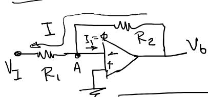
$$I = \frac{V_o - V_A}{R_2} = + \frac{V_A - V_I}{R_1} \Rightarrow \frac{V_o}{R_2} = - \frac{V_I}{R_1} \Rightarrow$$
