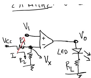
$$V_x = \frac{R_2}{R_1 + R_2} V_{cc}$$
