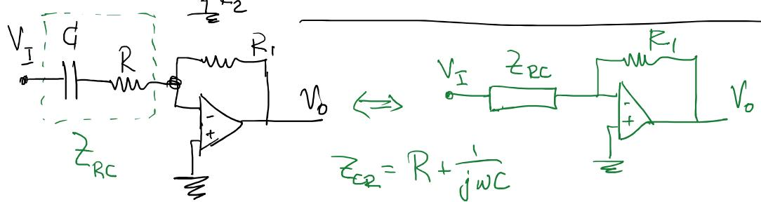
$$\frac{V_o(\omega)}{V_i(\omega)} = -\frac{R_1}{Z_{RC}} = -R_1 \frac{1}{R + \frac{1}{j\omega C}} = \left( -\frac{R_1}{R} \right) \frac{1}{1 + \frac{1}{j\omega CR}} \Rightarrow$$
