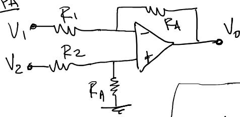
$$V_O = \frac{R_A}{R_2} V_2 - \frac{R_A}{R_1} V_I$$
