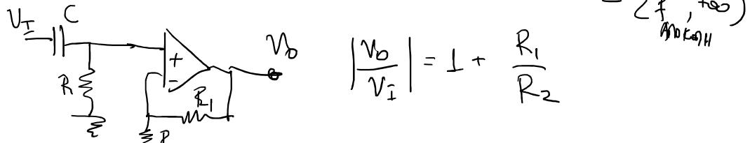
$$\left| \frac{V_o}{V_i} \right| = 1 + \frac{R_1}{R_2}$$
