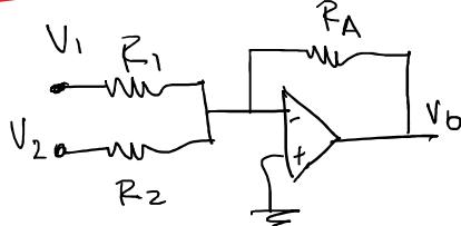
$$V_O = -\frac{R_A}{R_1} \cdot V_I - \frac{R_A}{R_2} \cdot V_2$$
