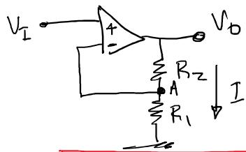
$$I = \frac{V_O - V_A}{R_2} = \frac{V_A}{R_1} \Rightarrow \frac{V_O - V_I}{R_2} = \frac{V_I}{R_1} \Rightarrow$$
