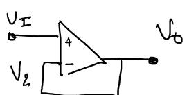
$$V_2 = V_o \Rightarrow V_o = V_I \Rightarrow G = \frac{V_o}{V_I} = 1$$
