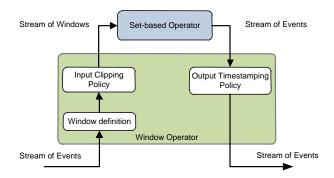
Figure 7. Input clipping and output timestamping policies.
