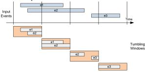
Figure 8: Tumbling windows with fully clipped events.
