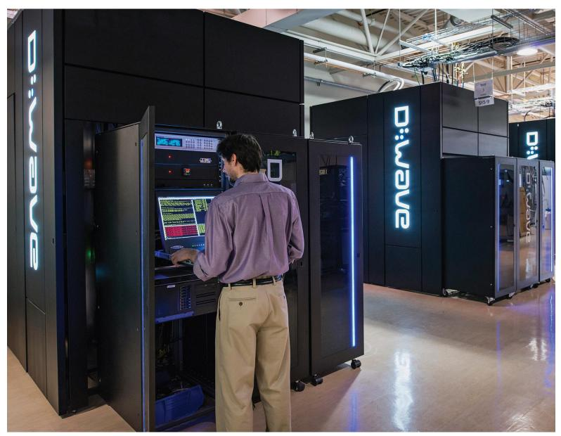
Reducing the temperature of the quantum processor to near absolute zero is required to isolate it from its surroundings so that it can behave quantum mechanically.
