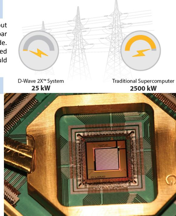
The D-Wave 2X system is based on a fabric of 1000+ qubits and over 3000 couplers. In order to attain this scale the processors contain over 128,000 Josephson Junctions - believed to be the most complex superconductor integrated circuits ever built.
