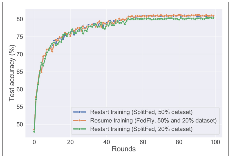
FIGURE 4. Global accuracy when 20 percent and 50 percent of datasets are required for training on a mobile device for 100 rounds of training.
