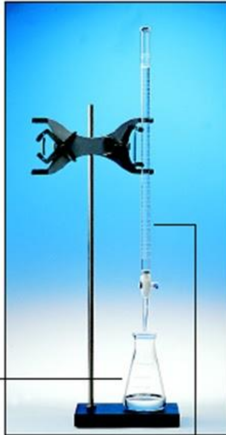
(a) 50-mL buret containing aqueous NaOH of accurately known concentration
