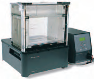
Fig 3. Ettan DALTwelve Large Vertical System.
