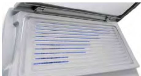
Fig 28. Example of IPG strips in a Reswell Tray.
