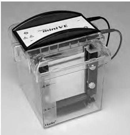
Fig 4. miniVE Vertical Electrophoresis System.
