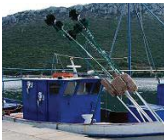
Figure 11(c): Reflectors used to enable the localization of the surface purse seine (Photo:V. LEKKAS).
