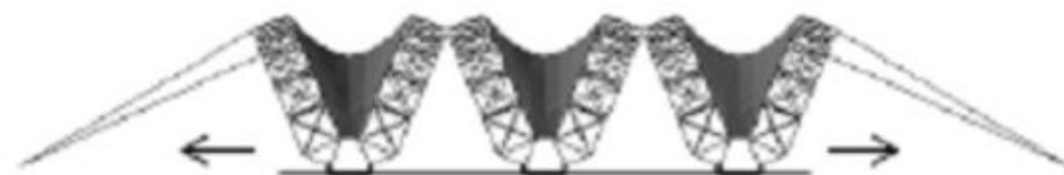
(b) Arches are slid along ground beam
