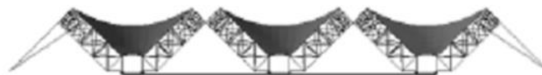
(c) Membrane is stretched to final configuration
