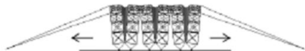
(a) Arches are installed upright
