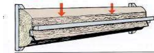
Flat slicing A common method for producing traditional crown-cut veneers.
