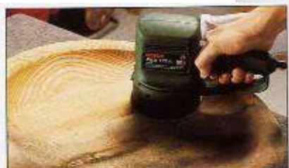
Keep the tool moving while sanding a workpiece.
