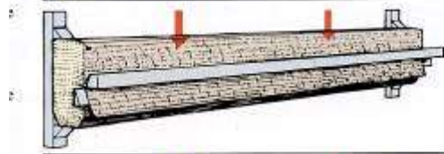
Quarter-cut slicing Used to produce veneers displaying attractive quarter-cut figure.
