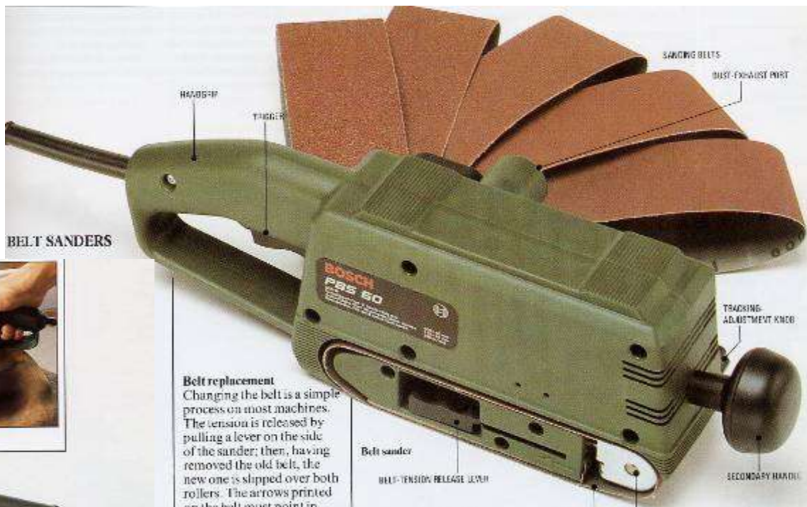
Keep the tool moving while sanding a workpiece.
