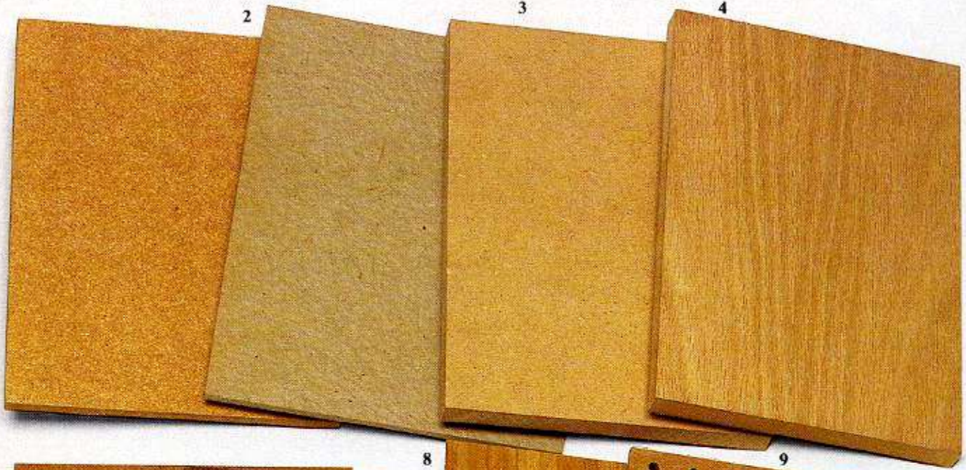
Medium boards 1 High-density (HM) board 2 Low-density (LM) board 3 Medium-density fibreboard (MDF) 4 Oak-veneered MDF board
