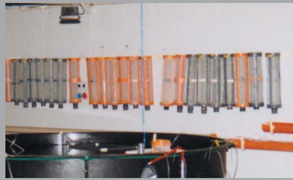
Fig.48.03-4-5-6 Larval rearing screen outlet changing, washing, disinfecting and stocking (photo STM Aquatrade)
