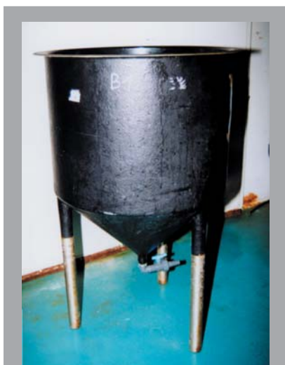
Fig. 43.00 Fiberglass cylindroconical tank used for eggs incubation (photo STM Aquatrade)
