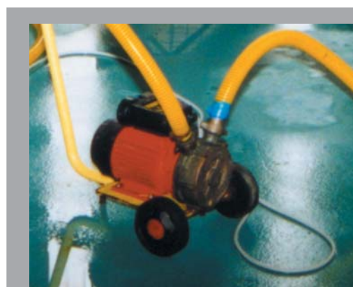
Fig.52.04 Wine reversible pump used to transfer live food (photo STM Aquatrade)
