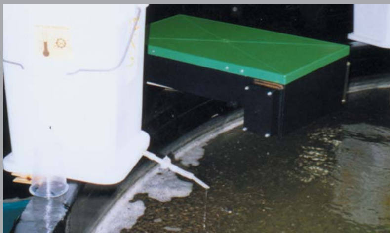
Fig.51.01 Belt feeder and the Artemia nauplii dispenser during gilthead sea bream weaning (photo STM Aquatrade)
