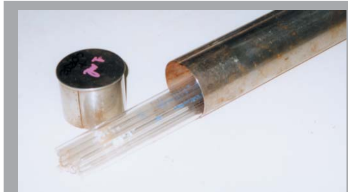
Fig. 24.05 Pipette container used with oven sterilization (photo STM Aquatrade)
