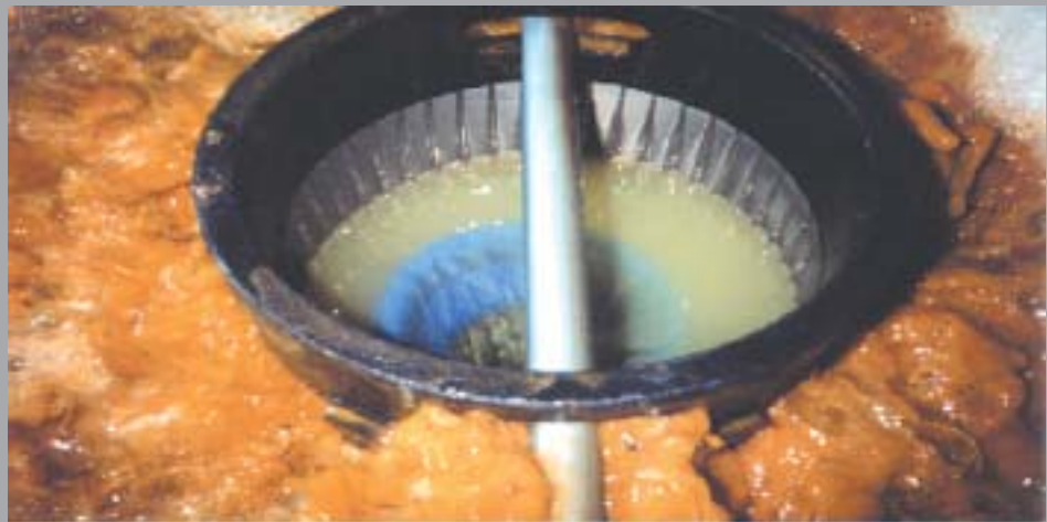
Fig. 36.01-2-3-4 Artemia industrial decapsulation (photo INVE Aquaculture)
