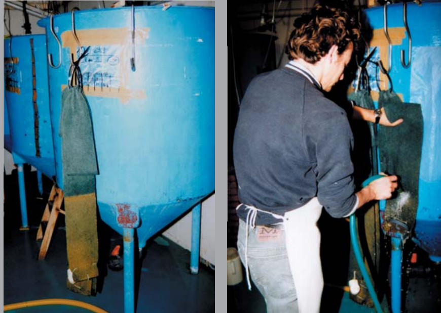
Fig. 31.01-2 Scotch Brite™ after one night of work and during cleaning procedures (photo STM Aquatrade)
