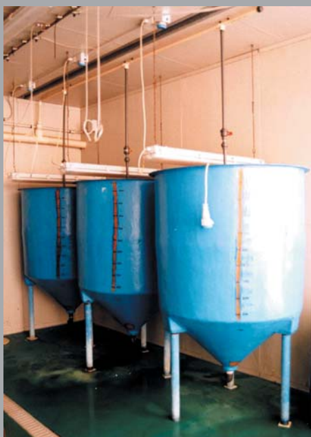
Fig. 37.01 Artemia incubation tanks of 1 m 3 (photo STM Aquatrade)
