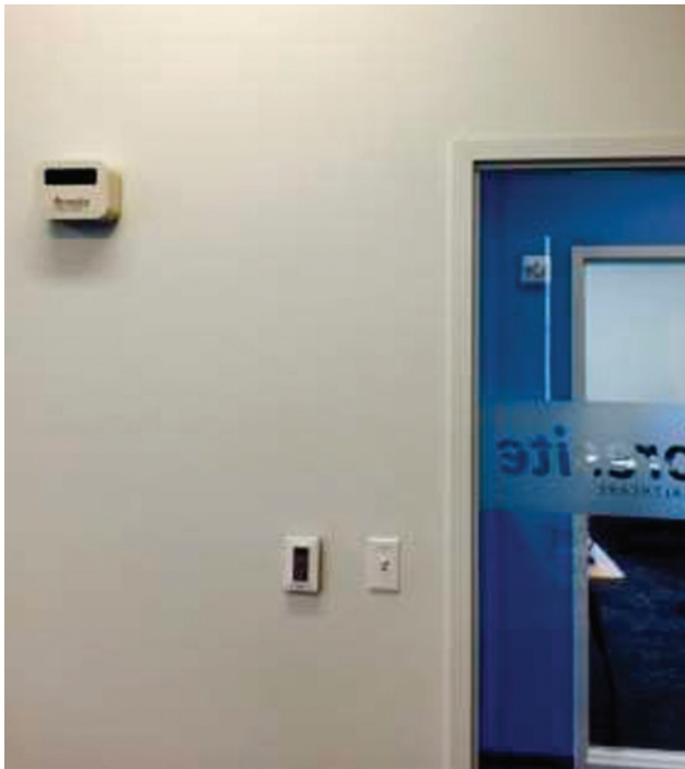
Figure 1. The integrated Foresite Healthcare data logger computer and depth sensor unit, sized at 5 × 7 × 3 in. mounted on a wall.
