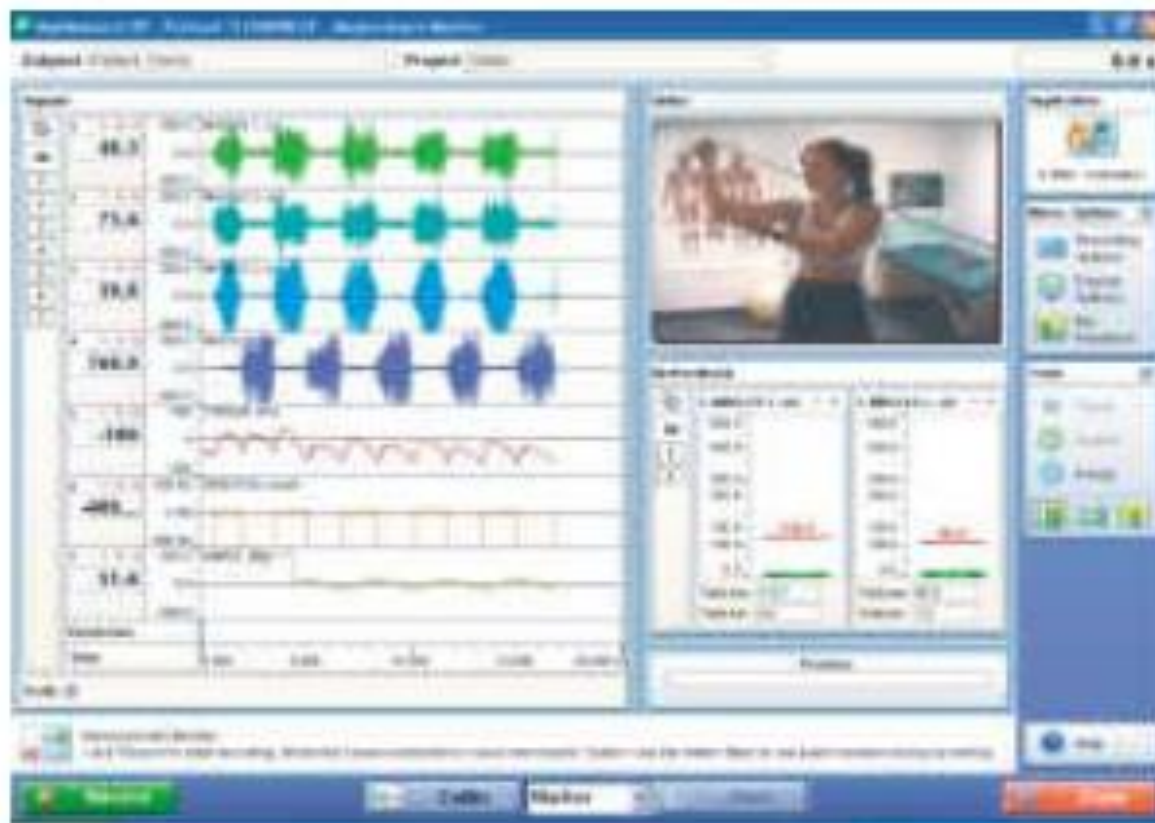
Fig. 4: Direct look into the body / muscle function: EMG synchronized with video and other movement sensors. Software screenshot of MyoResearch XP™ - NORAXON INC. USA
