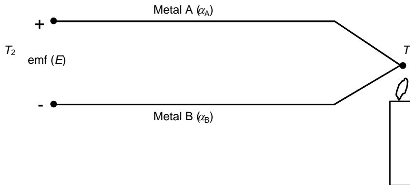
Figure 1. Schematic of a thermocouple made of metal A, with Seebeck coefficient \alpha_A , and metal B with Seebeck coefficient \alpha_B .
