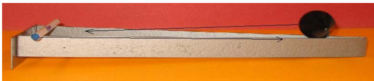
Figure 1. The double conic roller. The pen rolls down the incline from left to right. However, the double cone rolls from right to left, sinking inside the wedge.
