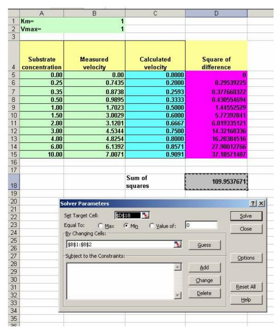
As you can see the Target cell is set to the sum of the square difference and it will be minimized by changing the cells which contain the random values of Km and Vmax.
