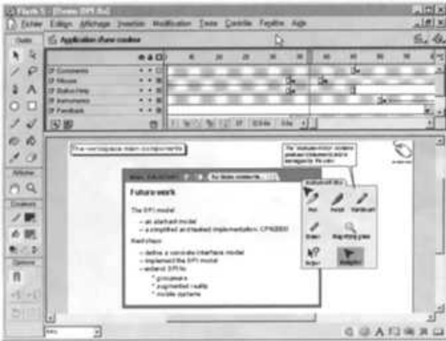
FIGURE 52.10. A noninteractive simulation of a desktop interface created with Macromedia Flash. The time line (top) displays the active sprites and the main window (bottom) shows the animation. Reprinted with permission from O. Beaudoux.
