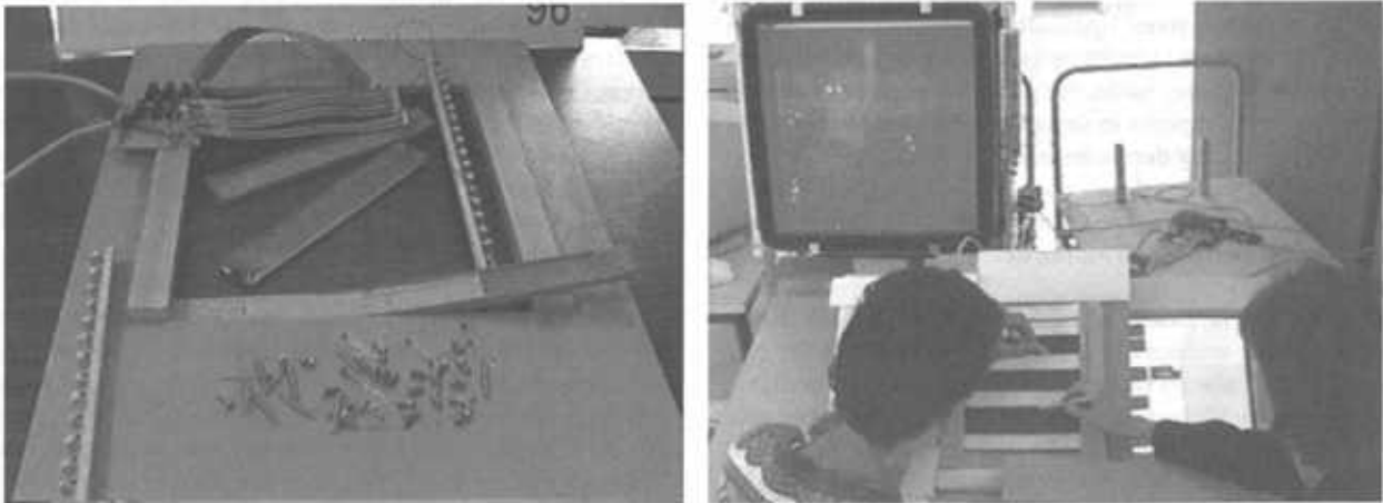
FIGURE 52.16. Caméléon's augmented stripboard (left) is a working hardware prototype that identifies and captures hand writing from paper flight strips. Members of the design team test the system (right), which combines both hardware and software prototypes into a single interactive simulation.
