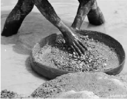
Worker hand-processes stream gravels of a placer deposit in search of diamonds. Image by USAid.gov.
