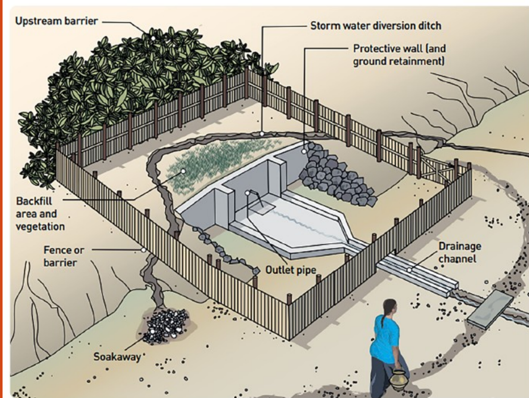
Gravity overflow spring. Source: SMET & WIJK (2002)
