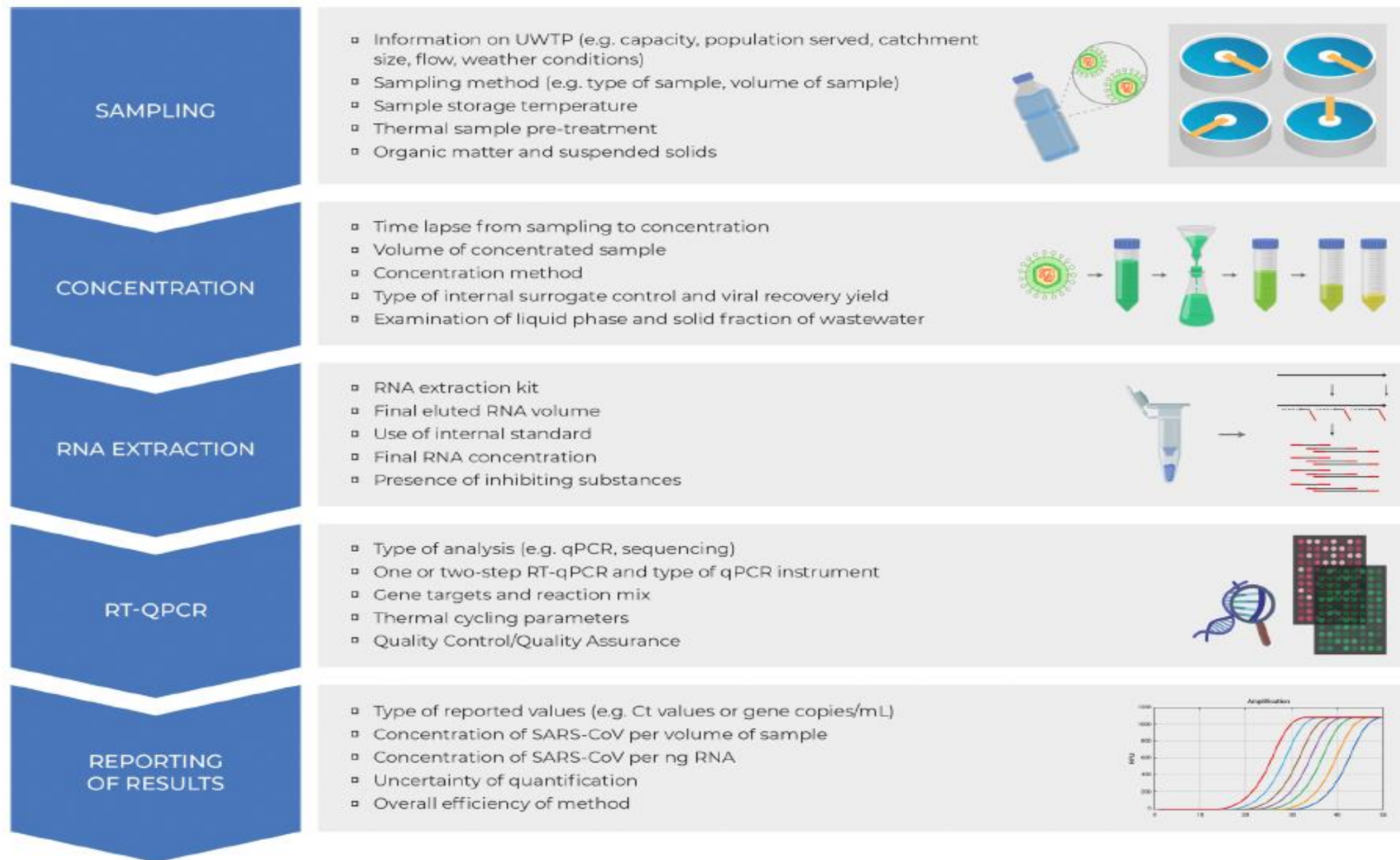
Fig. 1. Suggested key points according to each process step of the SARS-CoV-2 methodology for consideration.
