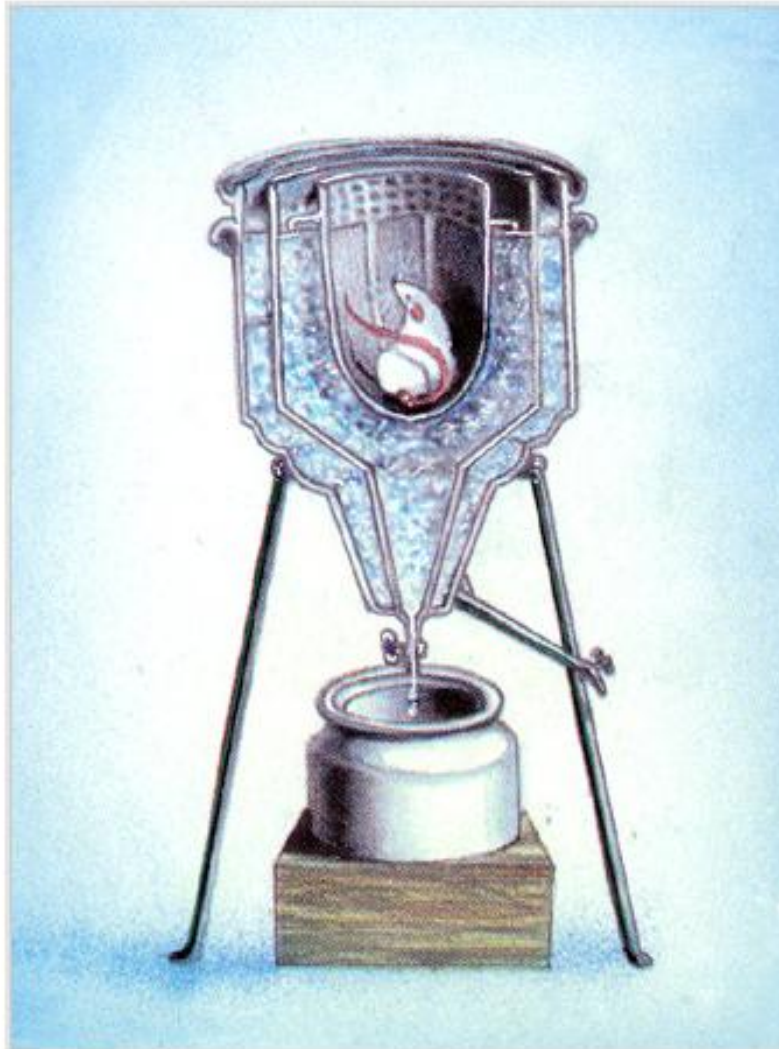
Ice calorimeter developed by Lavoisier and Laplace
