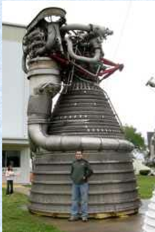
F-1 Engine Saturn V 1.5 million lbs thrust (SL) LOX/Kerosene
