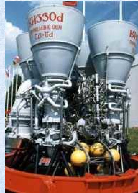
RD-170 1.78 million lbs thrust (SL) LOX/Kerosene
