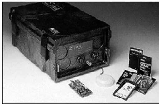
Figure 5.14. Example of a recorder made specifically for strong motion, the Kinematics Etna. The round white box in front of the recorder is the GPS antenna and the PCMCIA cards are seen to the right. From Kinematics home page www.kinematics.com .
