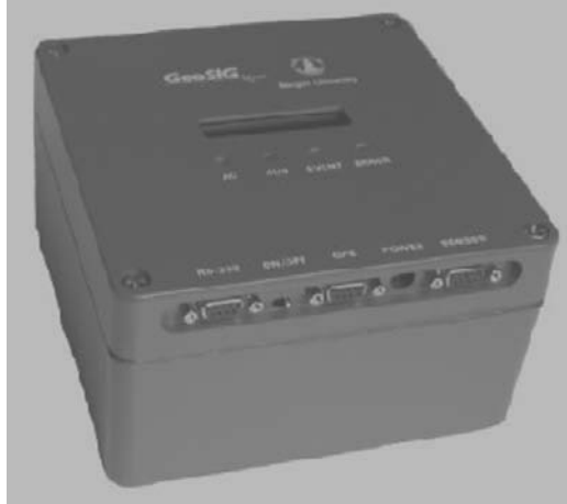
Figure 5.12 The GeoSIG compact seismograph with 3 built in 4.5 Hz sensors. Note the standard computer connectors. In the middle on the lid is located a display giving alphanumerical information and 4 LED's give operational information. This is the most compact complete seismograph on the market. Figure made available by Christoph Kündig, GeoSIG.
