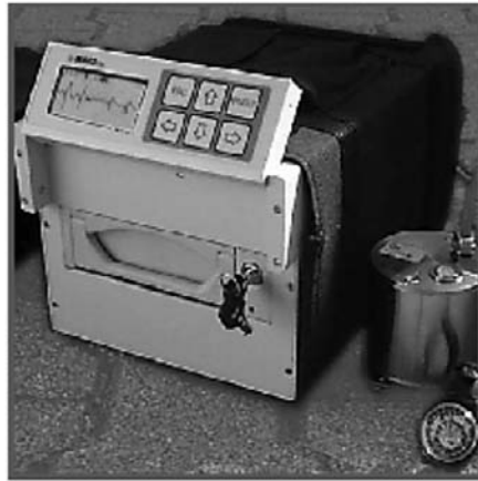
Figure 5.11. The Lennartz MARSliteHD recorder. Below the display is seen the 3.5" extractable hard disk. The model with magneto-optical recording is less than half the size (bottom part missing). From Lennartz home page, www.lennartz-electronic.de .
