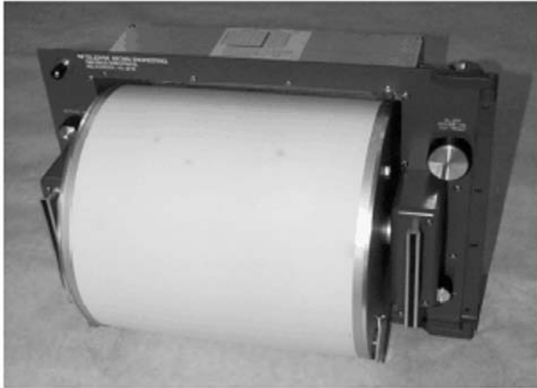
Figure 5.4 An example of a helicorder. The unit consists of a rotating drum with paper and a pen mounted on a pen motor that translates from left to right as the drum rotates. The gain of the pen amplifier is variable to adjust to different noise conditions. This recorder is made by Geotech (Model Helicorder RV-301B). From Geotech home page, www.geoinstr.com .
