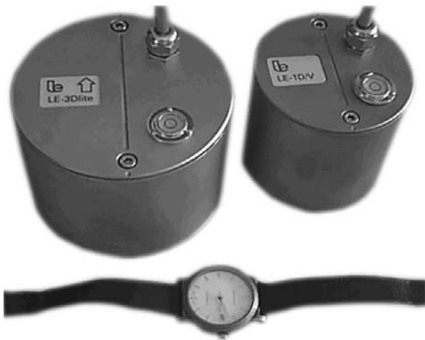
Figure 2.46 The Lennartz negative feedback 3 (left) and 1-component sensors based on 4.5 Hz geophones. From www.lennartz-electronic.de .
