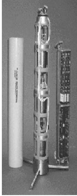
Figure 2.47 A BB borehole sensor model KS-54000 from Geotech Instruments. The height is 2.5 m. From www.geoinstr.com .
