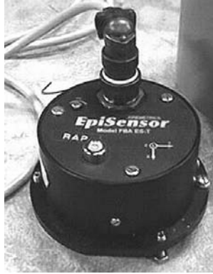
Figure 2.43 The Kinometrics EpiSensor. The case contains a 3-component sensor. The diameter is 13 cm.
