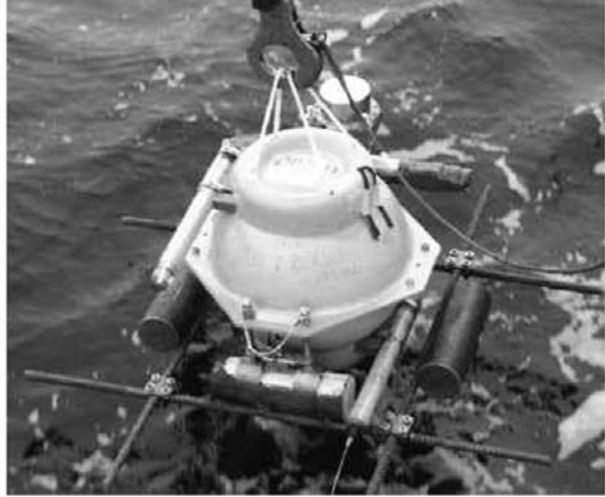
Figure 5.10 Example of an OBS. To the left is shown the key elements of the OBS and to the right is seen an OBS starting its journey to the bottom of the ocean. A flasher light is attached to the left side, a radio beacon to the right and the acoustic release equipment to the rear side. The metal bars on the bottom are the anchor left on the bottom after deployment. This OBS was developed at the Hokkaido University, Institute of Seismology and Volcanology, Japan. Figure from Department of Earth Science home page, www.geo.uib.no .
