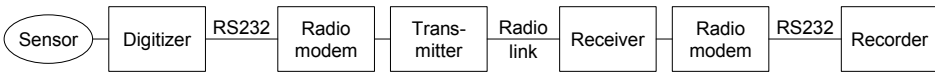
Figure 8.19: One way communication from a remotely installed digitizer via a digital radio link to a centrally located PC. The radio modem and transmitter /receiver might be one unit.
