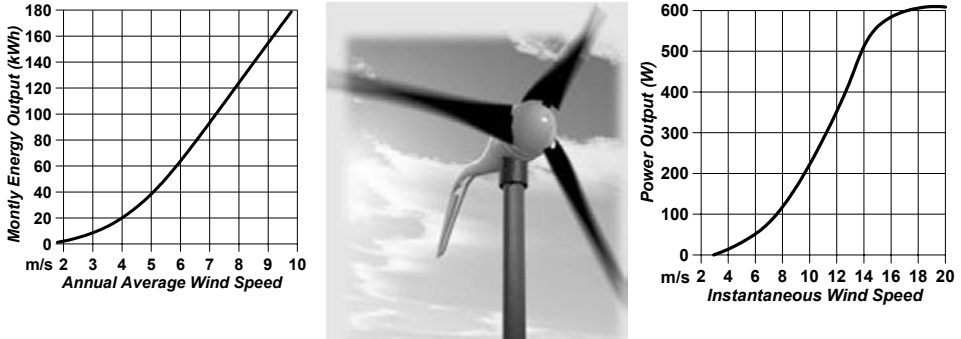
Figure 7.16 The Air 403 wind generator. To the left is shown the monthly energy output as a function of average wind speed. To the right is shown the power output as a function of the instantaneous wind speed (Figure modified from Southwest Windpower, www.windenergy.com ).
