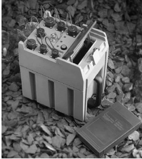
Figure 5.13 The Earth Data PR6-24 recorder. The length is 25 cm. Figure made available by Tony Russell, Earth Data.
