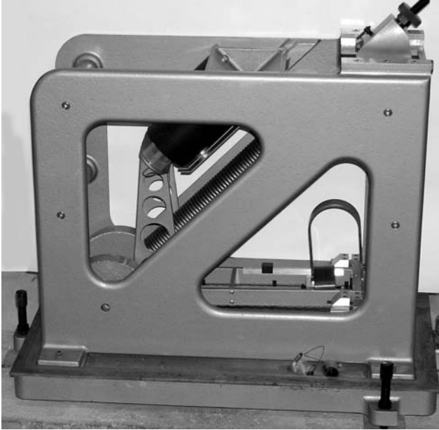
Figure 2.18 A typical vertical long period seismometer made by Sprengnether. The cylinder seen at top center is the magnet and the coil is moving with the mass seen bottom left. Leveling is done with the 3 screws at the corners of the base plate. Once the horizontal leveling is done (back screws), the front screw is used to adjust the period. The base plate side length is 60 cm and the weight 50 kg.
