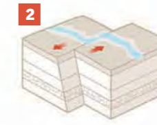
2 Displaced Streambed The streambed looks "broken" along its fault line.
