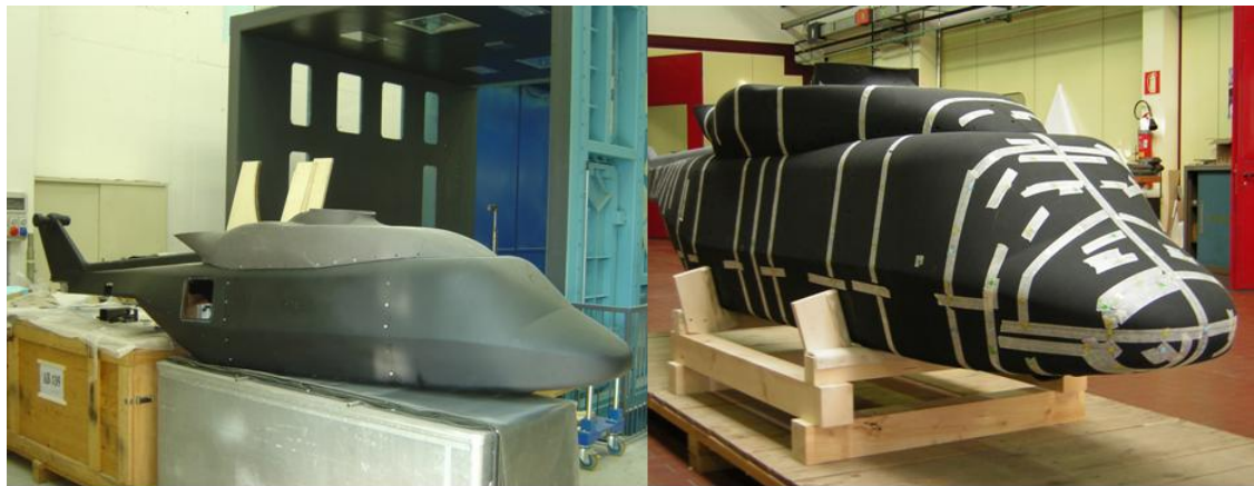
location of pressure sensors and hot films (14 June 2006)
