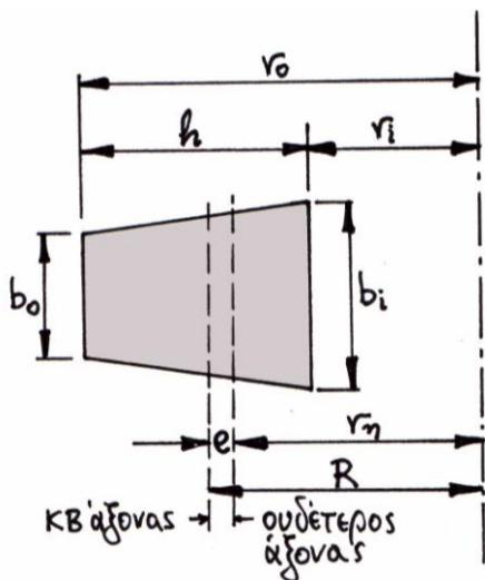
$$r_n = \frac{\left(\frac{b_i + b_o}{2}\right)h}{\left(\frac{b_i r_o - b_o r_i}{h}\right) \ln \frac{r_o}{r_i} - (b_i - b_o)}$$
