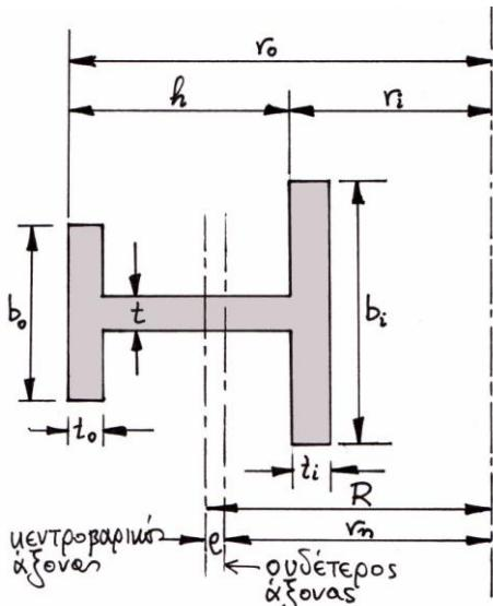
$$r_n = \frac{t_i(b_i - t) + t_o(b_o - t) + th}{b_i \ell n \frac{r_i + t_i}{r_i} + t \ell n \frac{r_o - t_o}{r_i + t_i} + b_o \ell n \frac{r_o}{r_o - t_o}}$$
