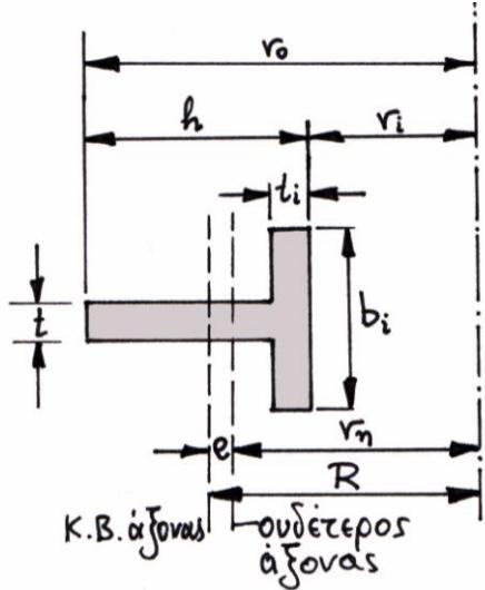
$$r_n = \frac{t_i(b_i - t) + th}{(b_i - t) \ln \frac{r_i + t_i}{r_i} + t \ln \frac{r_o}{r_i}}$$
