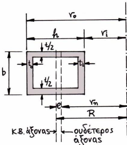
$$r_n = \frac{(b - t)(t_i + t_o) + th}{b \left[ \ln \frac{r_i + t_i}{r_i} + \ln \frac{r_o}{r_o - t_o} \right] + t \ln \frac{r_o - t_o}{r_i + t_i}}$$
