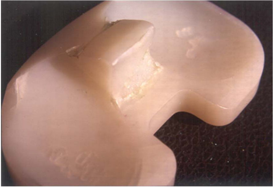
Fig. 6.41 Tibial Post and Bearing Wear.
