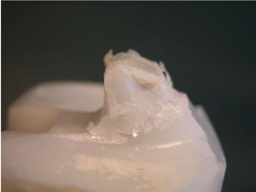
Fig. 6.42 Tibial Post Damage Due to Restriction in Axial Rotation in an IB Bearing.
