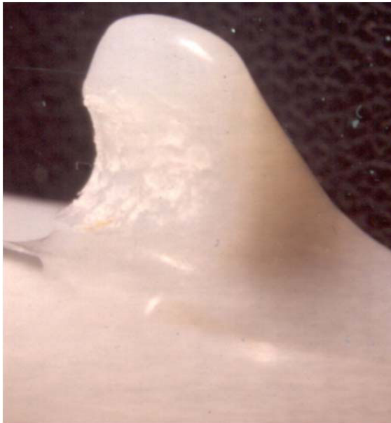
Fig. 6.40 "Wrap Around" Wear on a Post.
