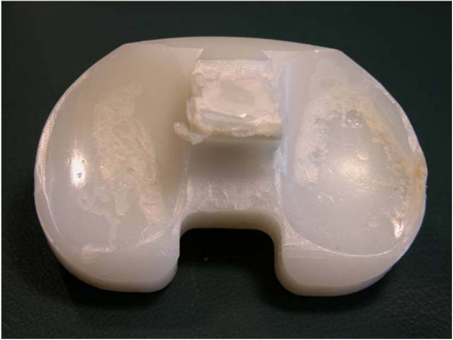
Fig. 6.43 Comparison of Post and Articular Surface Damage.
