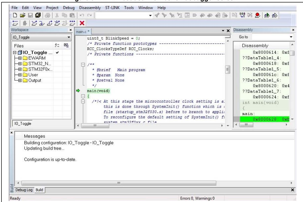
To run the application from the **Debug** menu, select **Go**. Alternatively, click the **Go** button in the toolbar to run the application (see [Figure 10](#)).
