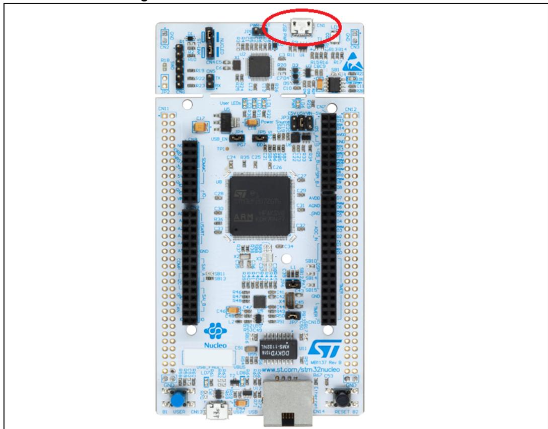
Figure 3. Connector CN1 for Nucleo 64 board
