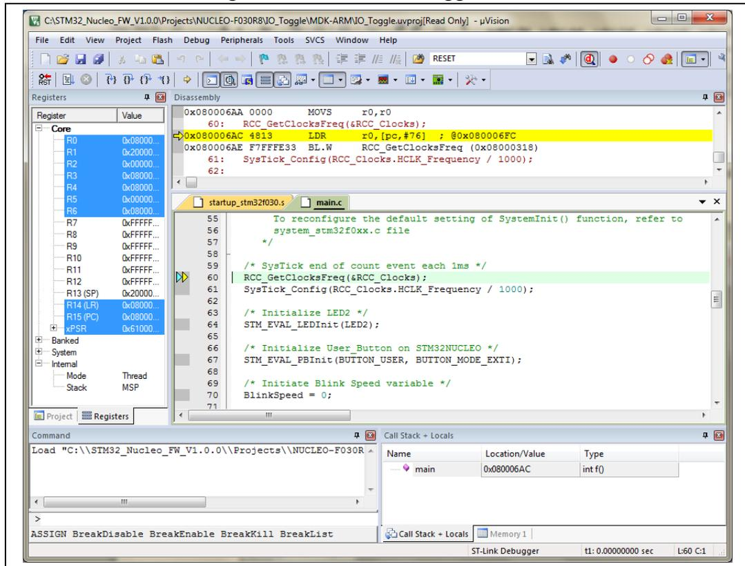
To run the application from the **Debug** menu, select **Run**. Alternatively, click the **Run** button in the toolbar to run the application (see [Figure 15](#)).
