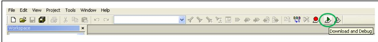
6. The debugger in IAR Embedded Workbench can be used to debug source code at C and assembly levels, set breakpoints, monitor individual variables and watch events during the code execution (see [Figure 9](#)).
