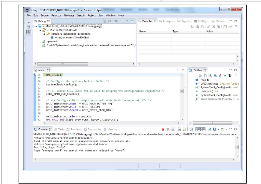
The debugger in the AC6 SW4STM32 can be used to debug source code at the C and assembly levels, to set breakpoints, to monitor individual variables and to watch events during the code execution.
